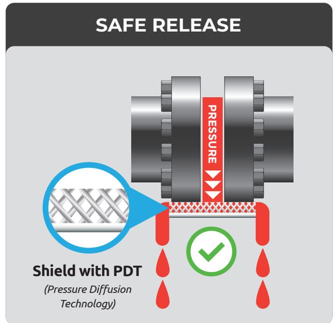
**SUREBAND® PDT (Pressure Diffusion Technology)** uses a specially formulated multi-layered mesh that is held against the flange. The pressure is diffused in a controlled manor thus preventing formation of a mist / vapour cloud. At the point of exit from the shield, the leak takes the form of a safe, vertical drip or stream.
